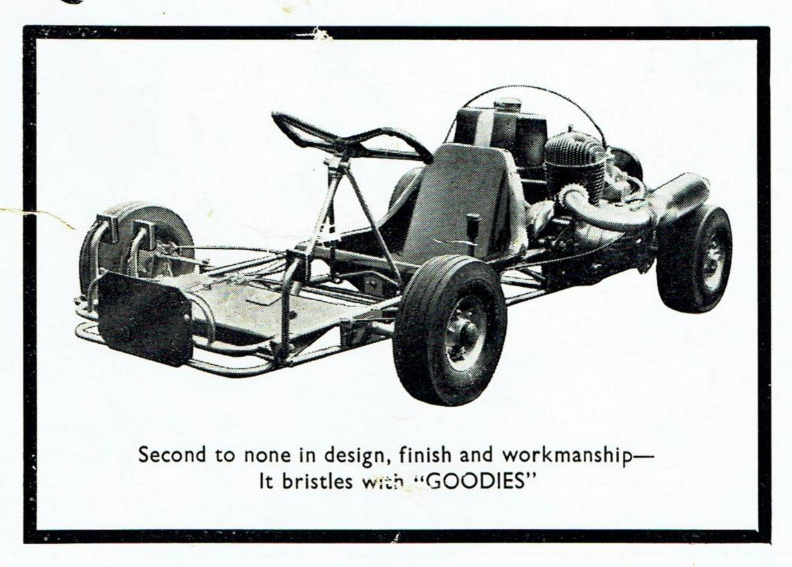
A The answer is the unique torque controlled flexibility of the chassis and the rigidity of the engine mounting.
