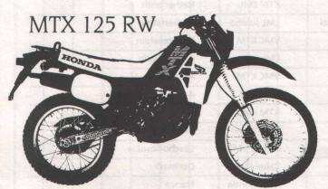
Liquid cooled 2-stroke single, competition styling, 6-speed transmission, CD ignition, and Pro-Link suspension.
