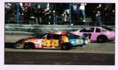
alike. These cars are exact 2/3 scale Nextel Cup replica cars imported from the USA. The cars feature a Baby Grand chassis, Yamaha FJ 1200 or XJR 1300 (1250cc) motorcycle engine, Winters Quick Change axle, lightweight fibreglass bodies, a single controlled slick and wet tyre, two types of shock absorber,
