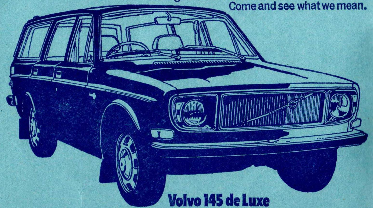
\*The little things (all standard features) 2-litre 4 cyl. 90 b.h.p. 5 bearing crankshaft engine. 67 cu. ft. (6' x 4') carrying capacity. Sealed cooling system. Alternator. Ignition and steering lock. Dual-circuit braking system. Reclining seats. Head restraints. Heated rear window with washer and wiper. Three-point safety belts. Hazard warning flashers. Laminated windscreen. Radial ply tyres. Anti-rust, hot-dip galvanised protection.
